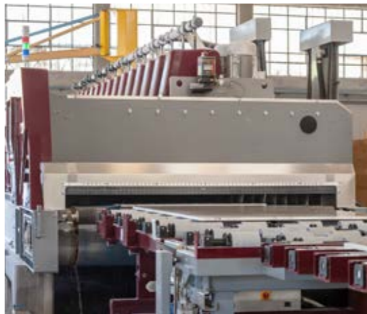
Particolare valvola guida lastre Detail of the slab centring valve
