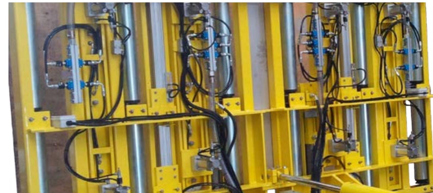
*The slab-loading/unloading trolleys automatically feed the material into the line.*
