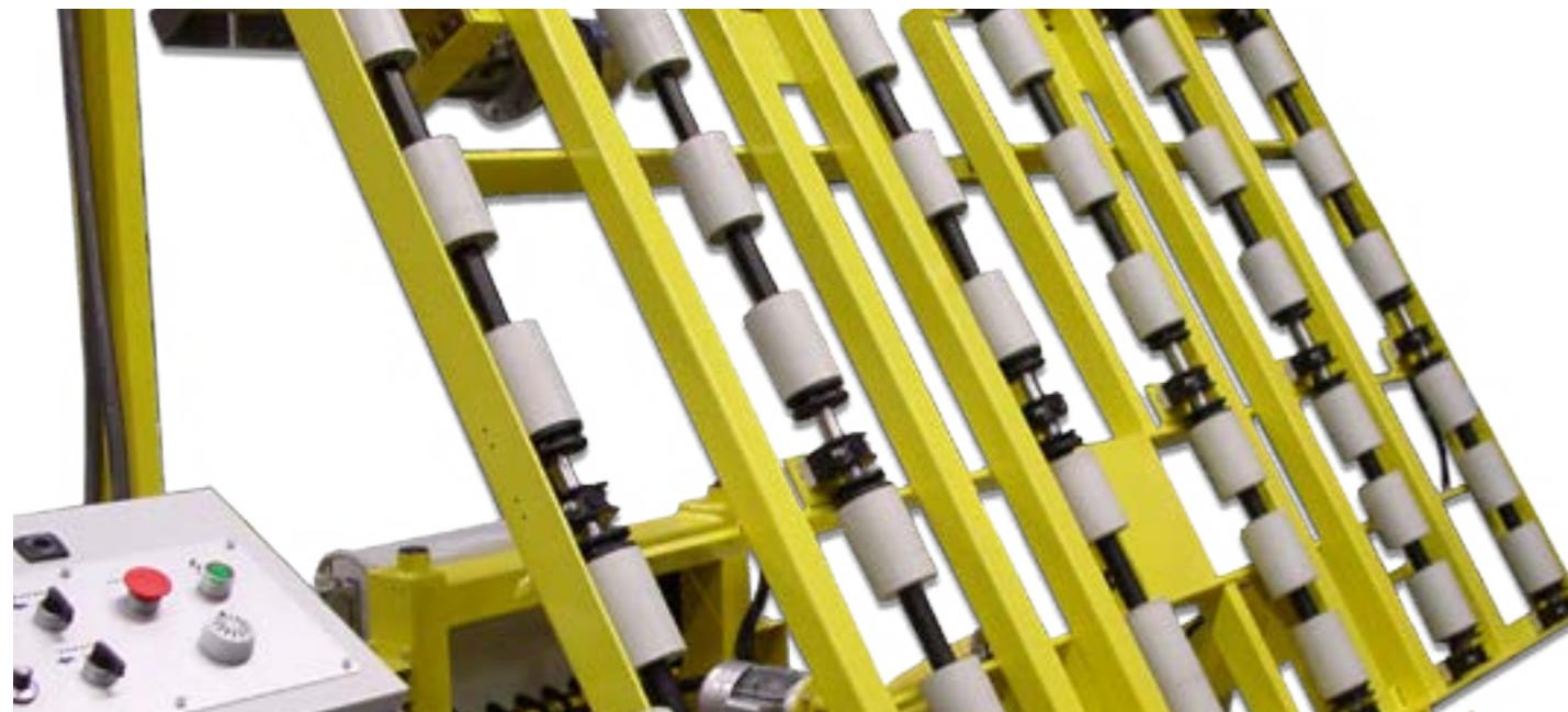
*One of the key components of reinforcement lines is the handling system, which must let the material move from one processing step to the next, quickly and safely. In some of CO.ME.S.'s plants specifically designed to treat extremely fragile slabs, the material is placed on the trays, gently taken through the entire process, and eventually ejected.*
