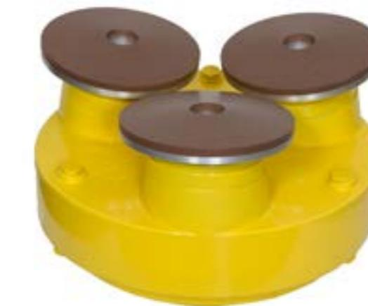
The "STORM" polishing machines are equipped with swinging arms heads, the result of years of experience working in the field. Extensive research into materials and tile processing techniques has led us to find the points that are key to the polishing process: the rotational speed of the head together with the frequency and oscillation amplitude of the foot are related to one another and this is key in providing the best possible performance ever.
