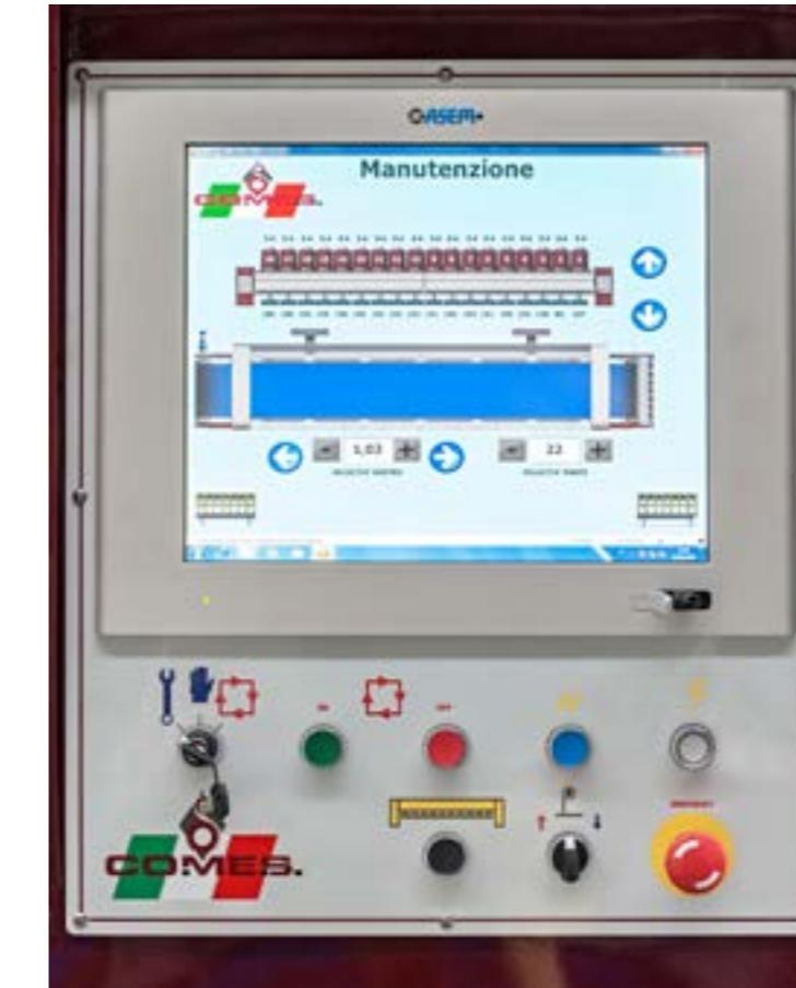
The electronics installed on the "STORM" polishing machine are both safe and powerful. Any function can be instantly retrieved on the user-friendly control panel, where you can easily adjust any setting as you like: belt speed, beam speed, deceleration at the edges of the slab, double polish in some places, etc. The machine has a touch-screen control panel with a colour graphic interface.
